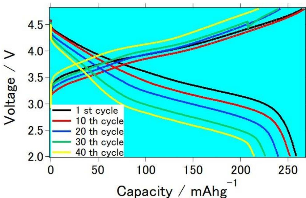
**Electrolyte : 1M LiPF<sub>6</sub> in EC / DEC (1/2) Potential window : 2.0 ~ 4.5 V**
